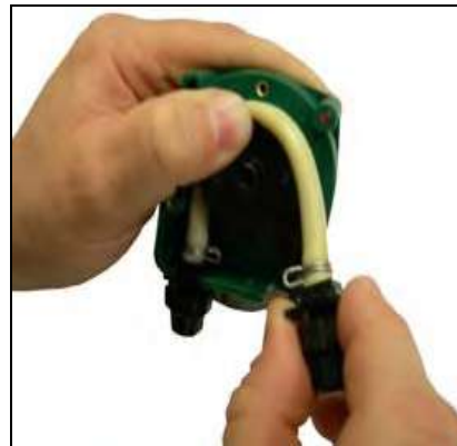
4. Hold the outlet fitting with one hand and with the other hand guide the tube into its position, reassemble the front cover with the screws provided.
