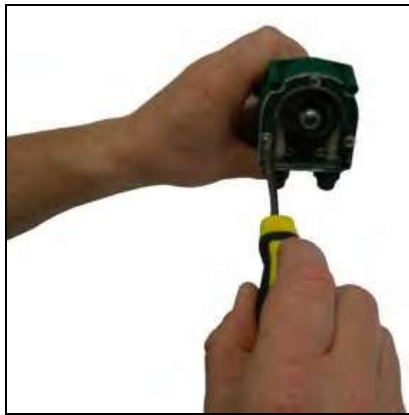
1. Unscrew the three cover screws using a Phillips screwdriver;
