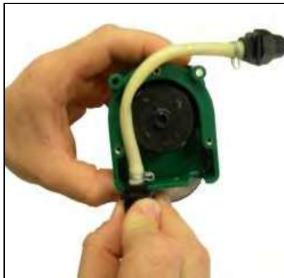
3. Replace with a new tube, after having lubricated the tube with silicon oil, and position the suction fitting into its slot;
