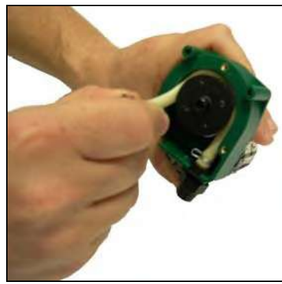
2. Extract the suction fixing and slide out the tube from the rotor in a clockwise sense;
